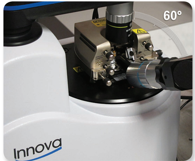
Optimized TERS configuration on Innova-IRIS.
