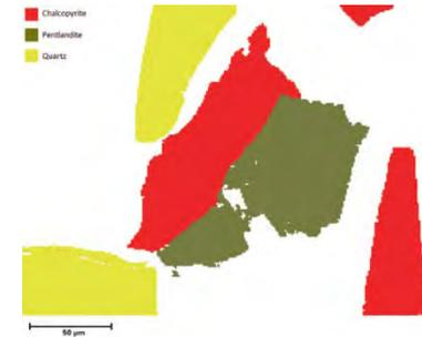
Resulting mineral map showing Chalcopyrite, Pentlandite and Quartz in Particle mode
