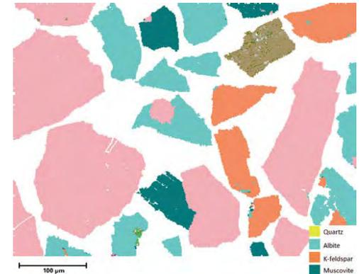
Resulting mineral map showing Quartz, Albite, K-feldspar and Muscovite after Particle mode analysis
