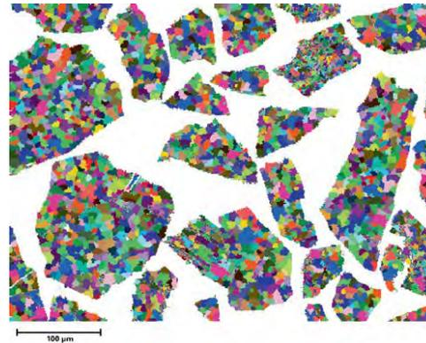
Particle segmentation image showing the result of segmentation of fine variations in BSE intensity
