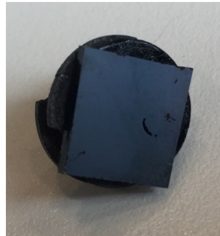
CIGS- wafer sample preparation for XRF analysis
