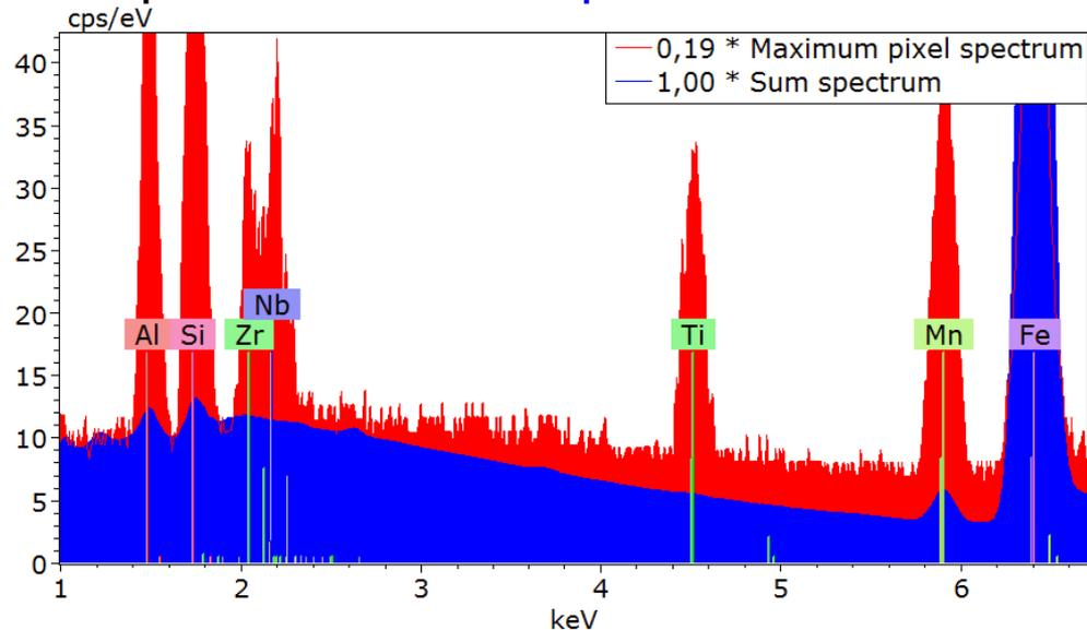
Niobium, zirconium and titanium had not been targeted by conventional wet-chemical analysis, but were identified by the Maximum Pixel Spectrum function.
