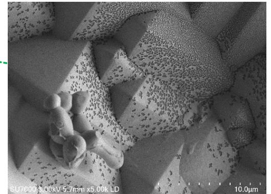
Specimen: Solar Cell incl. fluorescent material,  $V_{acc}$ : 3kV
