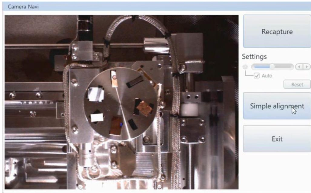
Automatically acquired picture of the sample holder and samples
