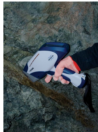
Measurements made with the Bruker Titan 800 handheld XRF
