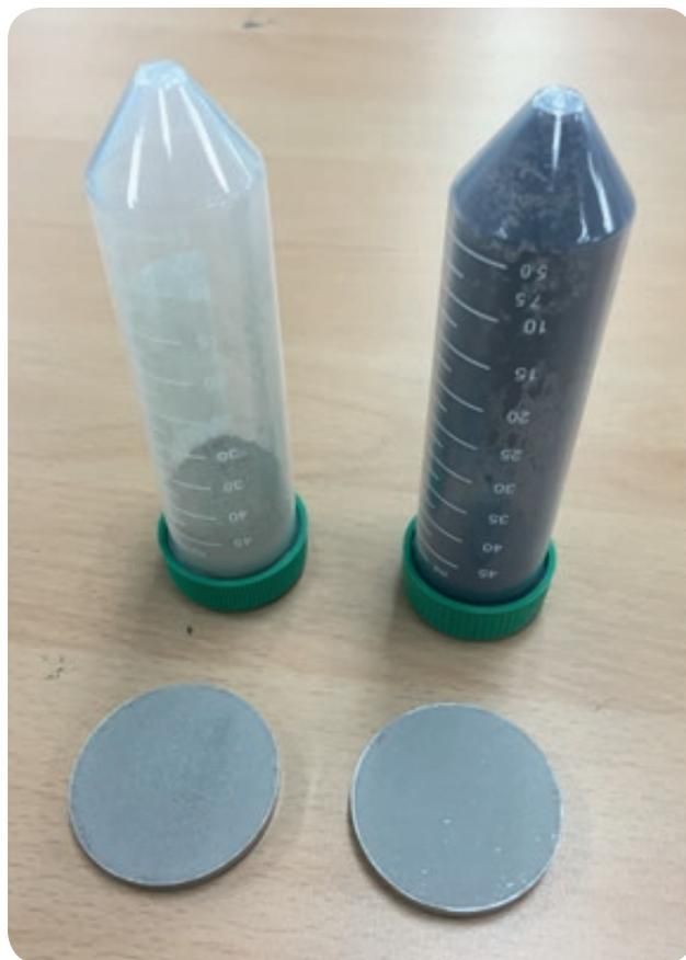
Figure 5: Raw sample material and prepared pressed pellets.
