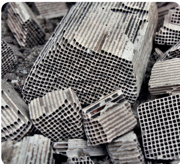
Figure 2: Typical monoliths from catalytic converters coated with PGE-containing films.
