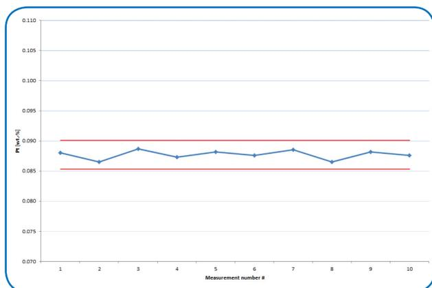
Figure 4: Excellent precision of Pt from the repetition test (see Table 3). Red lines denote  $3\sigma$  confidence interval.
