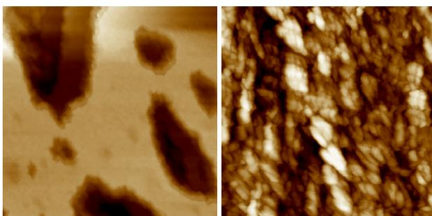
STM topography of template stripped gold (upper) and ITO (lower), 1µm x 1µm
