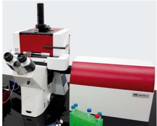
**Fig. 1:** The JPK NanoTracker™ 2 mounted on a Zeiss Axio Observer microscope. The trapping laser is coupled with a special side-port above the fluorescence filter wheel.
