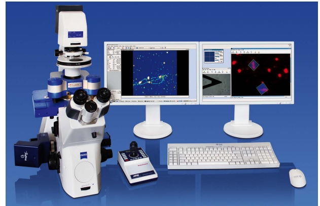
Fig. 1: NanoWizard® 3 AFM in combination with a Zeiss AxioObserver inverted microscope. Perfect integration is achieved by JPK's patented DirectOverlay™ approach.
