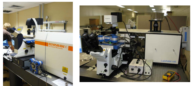
Fig. 2 Established example combinations of JPK NanoWizard® AFM and a JPK TAO™ module with Renishaw inVia and Horiba Jobin Yvon LabRam HR .
