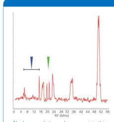
Nuclear resolution enhancement in this Davies ENDOR spectrum of a Cu-Pt complex facilitates assignment of nuclear couplings for the <sup>31</sup>P and <sup>195</sup>Pt
