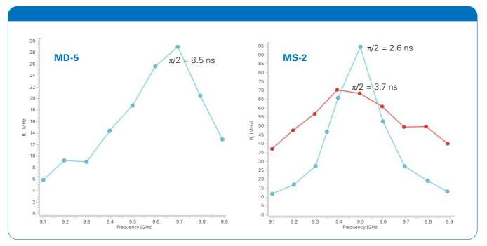
High B, and large bandwidth: Flexline bandwidth and B, at various coupling strengths (1 kW TWT)
