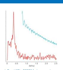
L-Band <sup>29</sup>Si –ESEEM. Increased modulation depth allows fewer averages for detection when compared to X-band.
