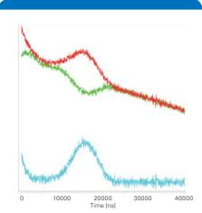
Nuclear spin FID and echo detection gives access to the nuclear spin relaxation times and provides additional filters for the ENDOR spectrum.
