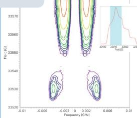
The higher g-value resolution at W-band provides the greater opportunities for orientation selective pulse experiments: 2D 4-pulse DEER experiment showing the parallel component of the dipolar spectrum with the pump pulse in the  $g_x$  region and the probe pulse in the  $g_y$  region.
