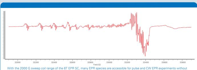
With the 2000 G sweep coil range of the 6T EPR SC, many EPR species are accessible for pulse and CW EPR experiments without changing the persistent field of the magnet.
