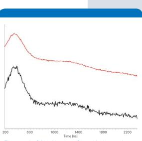
The superior S:N achieved at Q-band in the 4-pulse DEER experiment improves the reliability and accuracy of distances and distance distributions: Optimized sample amounts of spin labeled Ubiquitine, 10 µl at Q-band (red) and 150 µl at X-band (black).
