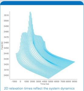
2D relaxation times reflect the system dynamics as related to the molecular structure: Echo decay (T<sub>2</sub>) vs Field of spin label encapsulated in Li-X.
