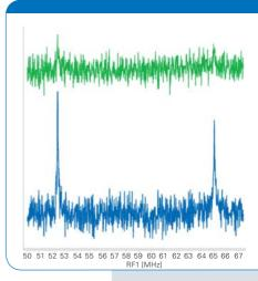
Linear sweep (top) and stochastic excitation (bottom) of <sup>31</sup>P nuclear spins in silicon at 10 K
