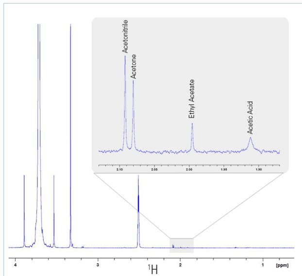
Identification and quantitation: The above  $^1\text{H}$  spectrum was acquired with the AvanceCore Foundation from a 20 mg sample in less than 5 minutes. The sample contains 100 ppm (0.002 mg) of the following impurities: acetonitrile, acetone, ethyl acetate and acetic acid in  $\text{DMSO-d}_6$ .
