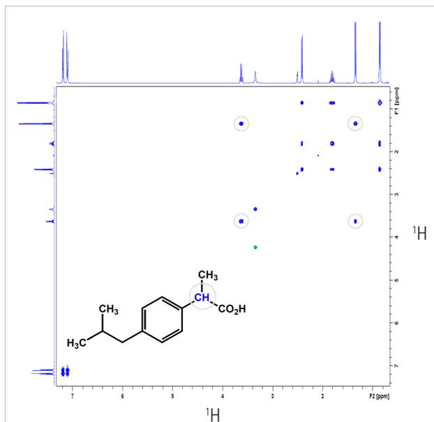
The AvanceCore Foundation also supports state-of-the-art  $^1\text{H}$ - $^1\text{H}$  2D experiments such as TOCSY, COSY, ROESY and NOESY. The above spectrum shows TOCSY-correlations of the anti-inflammatory drug Ibuprofen. The TOCSY can be used for structure assignment.
