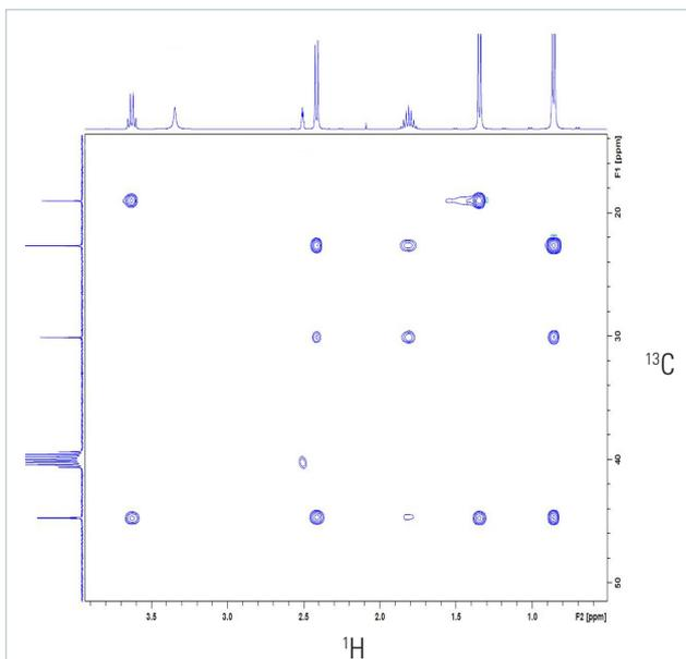
The AvanceCore Select supports heteronuclear experiments (HSQC, HMBC...) which are essential for molecular structure elucidation. The above spectrum shows a 2D  $^1\text{H}/^{13}\text{C}$  HSQC-TOCSY experiment recorded from a 20 mg Ibuprofen sample.
