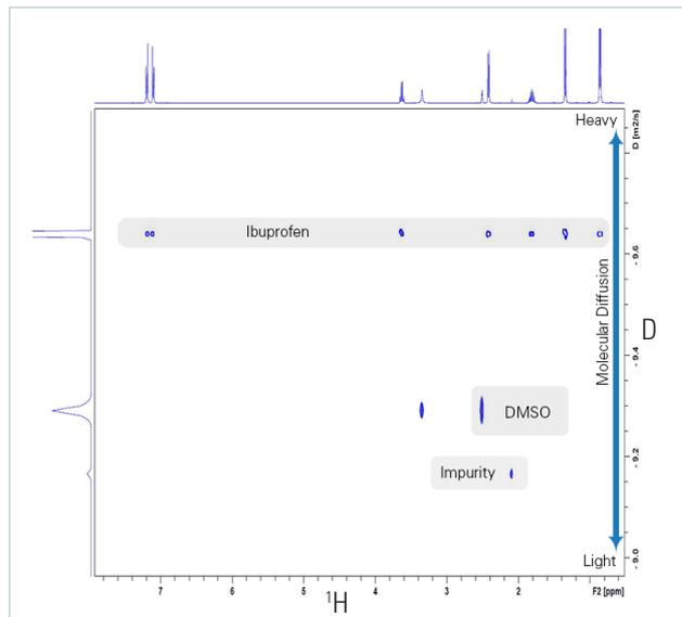
With the AvanceCore Foundation, the  $^1\text{H}$  DOSY NMR experiment for mixture analysis can be performed. DOSY is often referred to as “chromatographic NMR”. Just like LC-MS, it resolves the different mass and diffusion properties of individual mixture components.
