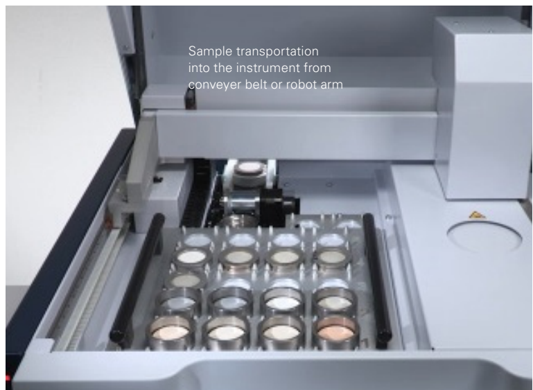
Insertion of sample into sample chamber directly or via buffer positions
