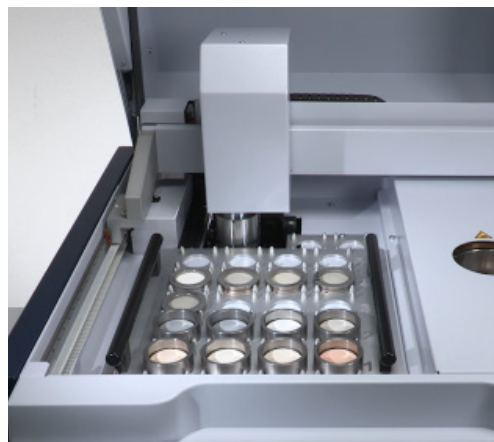
Insertion of sample into sample chamber directly or via buffer positions
