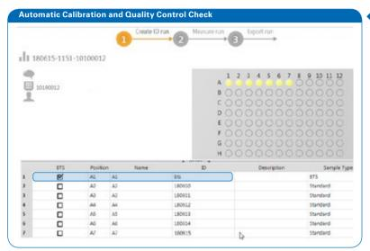
◆ The MALDI Biotyper System can automatically be checked by analysing Bruker Bacterial Test Standard (BTS) before each run. Using BTS for the quality control of the MALDI Biotyper assures the highest data reliability and measurement reproducibility.
