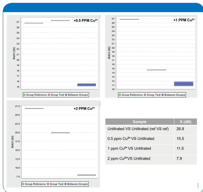
Figure 7. Statistical analysis (1D PROFILE) on the Fc-fusion protein supplemented with copper. Variability is quantified by the value S(dB), the logarithmic scale of similarity; 13,14 the higher the value, the higher the similarity. In all three statistical analyses (graphical plots), the variability between groups does not overlap with in-group variabilities, indicating statistically significant differences between spectra. In the table are reported the S(dB) value calculated for each sample when compared to the reference.
