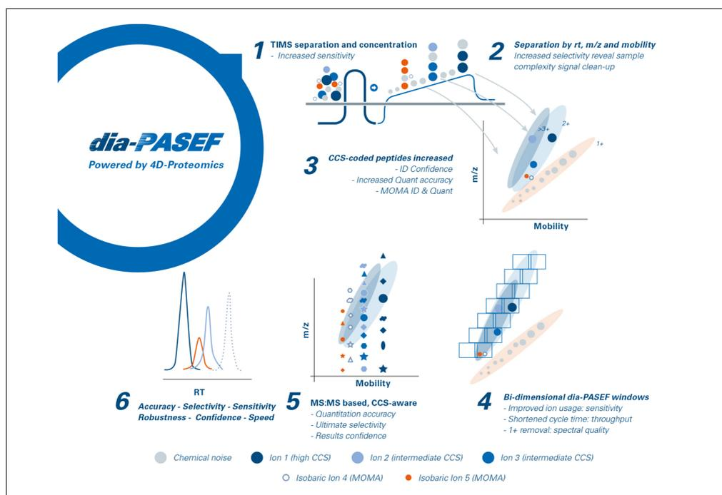
Fig. 1 dia-PASEF scheme of operation and advantages.
