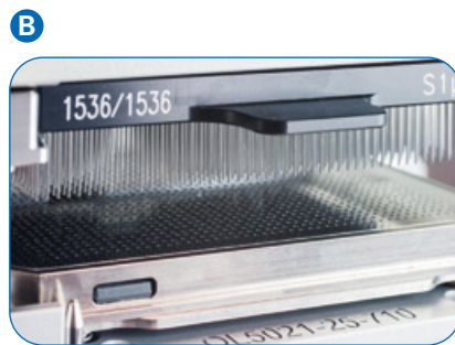
Figure 3. A CyBio® Well vario 1536 pipettor. B 1536 ceramic tips and 100nL matrix spotted on to a metal MALDI target. C Workflow detailing spotting/analysis process. (* dependant upon drying time).
