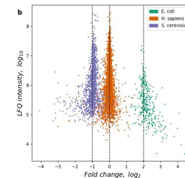
We performed benchmark measurements on a Bruker timsTOF Pro instrument with Parallel Accumulation Serial Fragmentation (PASEF) functionality for the acquisition of MS/MS spectra. We generated benchmark datasets in which HeLa proteins were spiked with E. coli and yeast proteomes at 1:4 and 2:1 ratios and compared the replicates with the MaxLFQ algorithm for label-free quantification.
