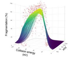
The collision energy used and fragmentation achieved in the testing set is shown in red, while the neural network prediction for varying collision energy levels of  $0\sim100$  eV are plotted in the Viridis color scale. The majority of the red dots fall close to the predicted model.
