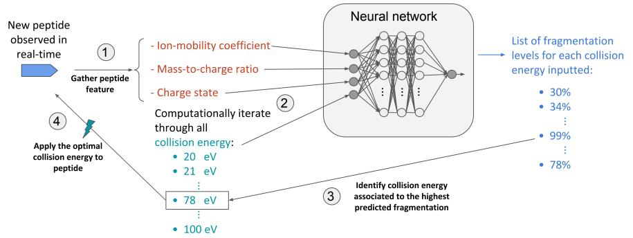
The optimal collision energy selection process could be executed under 5 ms on average, demonstrating capacity to be run in real-time during mass spectrometry.
