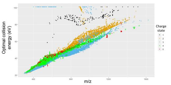
Predicted optimal collision energy v.s. m/z of a peptide, color-coded by charge
