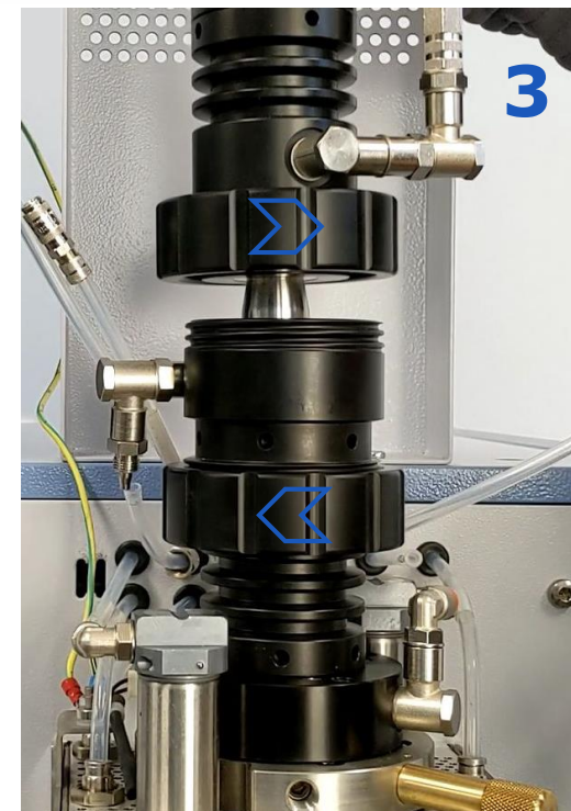
Removal of the autocleaner
