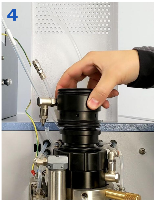
Removal of the filter
