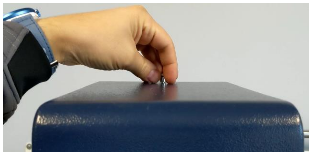
Loosening of the screws and removal of the protective cover
