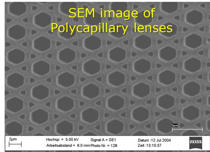
Poly-capillary lens collects large solid angle of tube radiation
