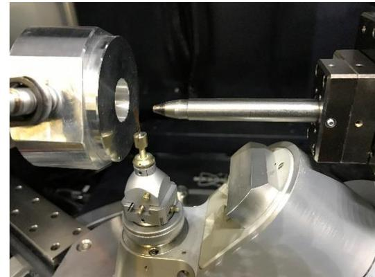
Pin diode mounted in front of the collimator
