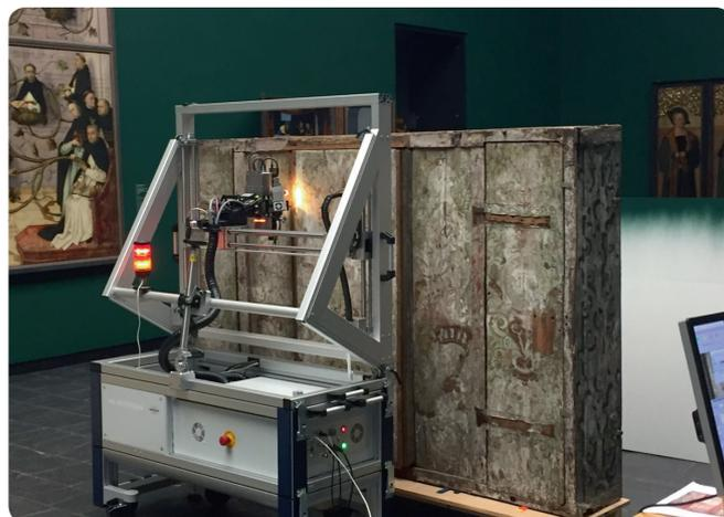
**M6 JETSTREAM™  $\mu$ -XRF analyzer**
