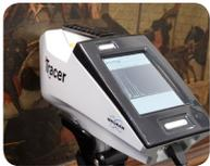
**Handheld XRF Elemental Analyzers:** *TRACER 5™ and S1 TITAN™ are the most agile XRF analyzers from Bruker Handheld XRF that simultaneously measure elements from sodium (Na) to uranium (U) at concentrations as low as parts-per-million to high percentage levels. These analyzers can be used on samples of any form (liquid, solid, powder, film) and analyzed at any location.*
