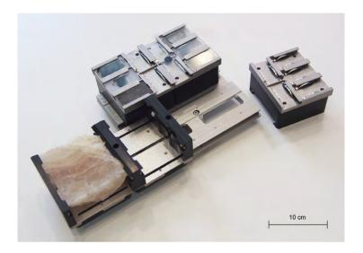
Optionally, there is an additional base plate, which supports drill core holders or thin section carriers. The drill core sample holder is configurable and can be adjusted to hold up to HQ sized (2.5 inch) drill cores. It can be set up with one or two halves, each of which can hold two or three half or quarter cores as well as end pieces or plugs. Alternatively, the base plate can be fitted with up to four thin section carriers, each being able to hold and secure five thin sections.
