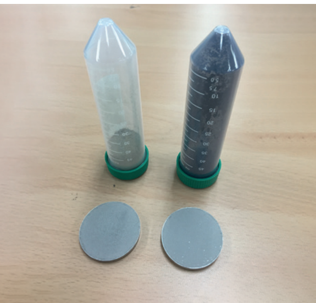
Figure 1 Typical monoliths from catalytic converters coated with PGE-containing films.
