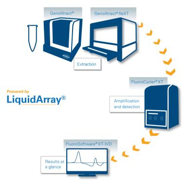
GenoXtract®: extraction 1-12 samples per run GenoXtract® fleXT: extraction and PCR setup for up to 192 samples per day
