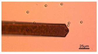
**Fig. 1**: Tipless cantilever in water with 5 µm micro-spheres
