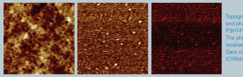
Topography (left), adhesion (middle), and photocurrent (right) of P3HT-PCBM. Image size 1µm. The photocurrent is seen to be localized in fibrils formed by P3HT. Data courtesy of Noham Sebaihi (CIRMAP – UMONS, Belgium).
