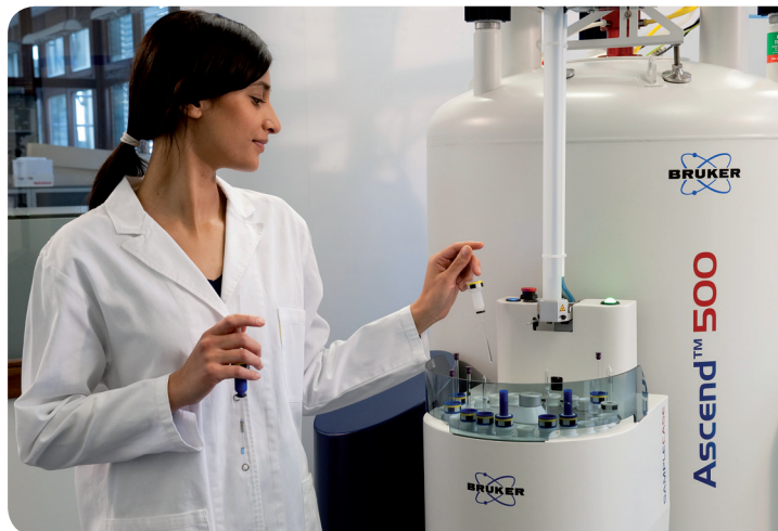
Ascend 500 equipped with SampleCase for easy automation
