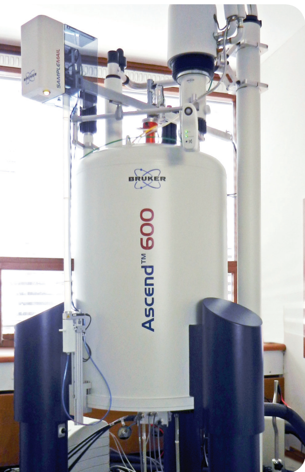
Ascend 600 with N 2 fill eliminating technology
