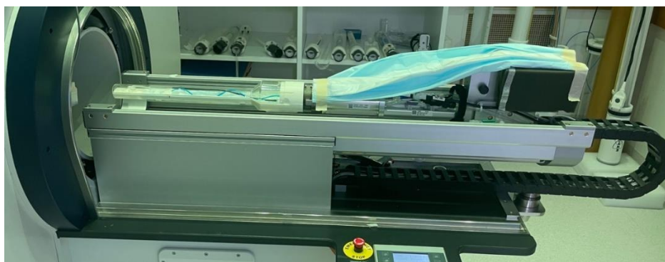
FIGURE 1. Bore of magnet showing the animal transport system known as Autopac and the MMPF cradle.
