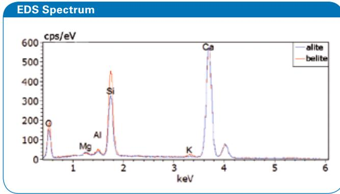
Fig. 1 Spectra of both calcium silicate phases
