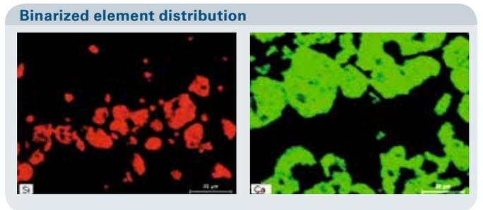
Fig. 4 Binarized element distribution of silicon and calcium
