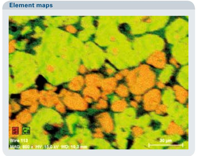
Fig. 3 Overlay of Si and Ca element maps (belite: orange, alite: yellowish green)
