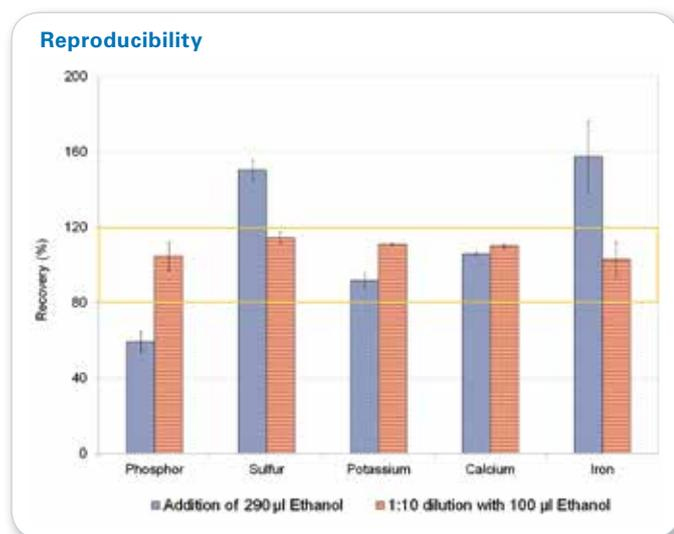
Fig. 4 Reproducibility of the measurement of nutrient elements in DMEM. The acceptable recovery limit of  $\pm 20\%$  is defined with the yellow frame.
