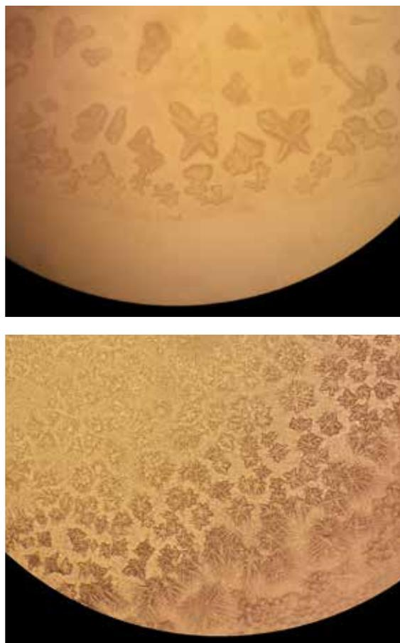
Fig. 2 10-fold magnified images of DMEM on quartz sample carriers after dilution with water (top) and ethanol (bottom).
