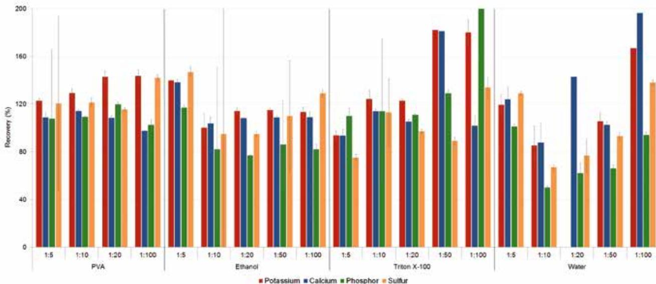
Fig. 3 Recovery of the nutrient elements K and Ca (measured with Mo-K excitation) and S and P (measured with W-L excitation) in DMEM with different smoothing agents and dilution factors.
