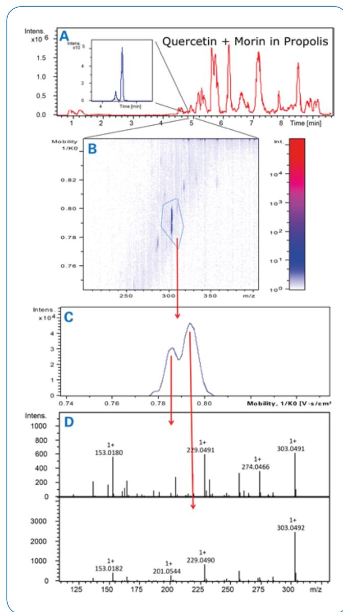
**Fig. 3:** **A** Base Peak Chromatogram and Extracted Ion Chromatogram of quercetin and morin of a propolis sample. **B** Heatmap of the area of interest. **C** Mobilogram revealing two isomeric compounds. **D** Clean MS/MS spectra after ion mobility separation.
