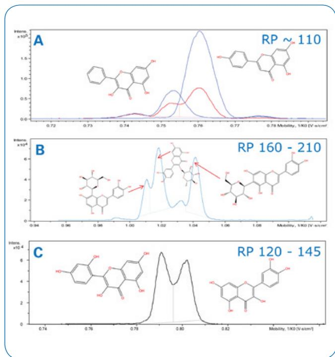
**Fig. 2:** Mobilograms of isomeric compounds showing ion mobility separation of mixtures. **A** Galangin and Apigenin, **B** Orientin, Isoorientin and Quercitrin, **C** Quercetin and Morin.
