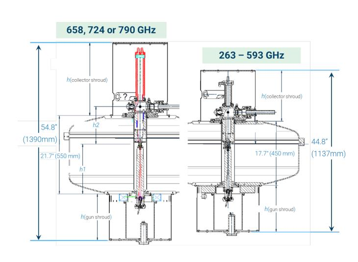
Cross-sectional view of Gyrotrons for up to 1.2 GHz (left), only 20 cm taller in the magnet stand and with matching diameter and footprint vs. to the 400 – 900 MHz family (right).
