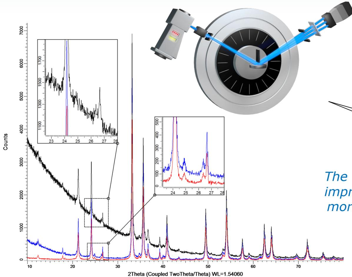
*The usage of a motorized knife improves the background even more, especially at low angles*
