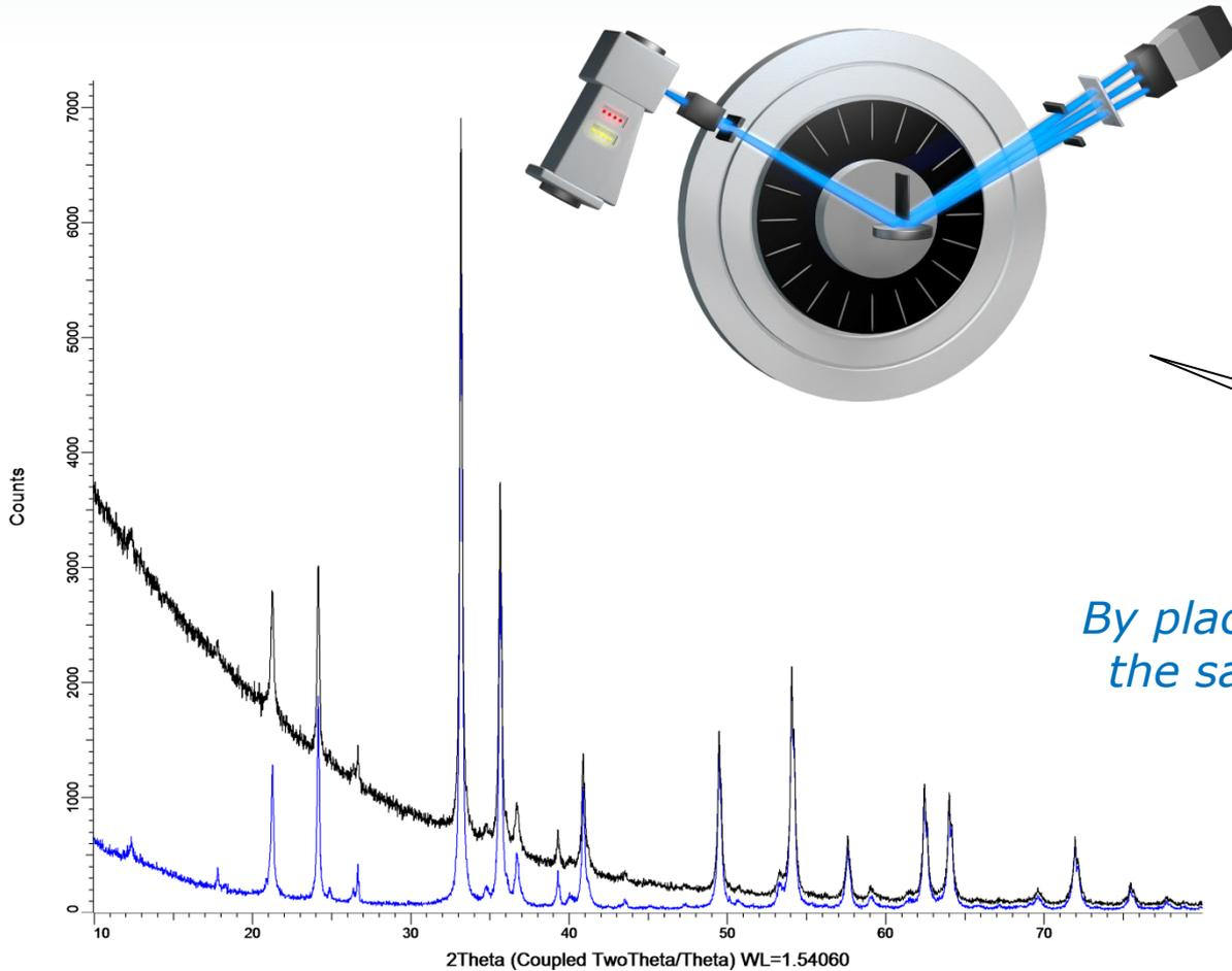
*By placing a fixed knife 5mm above the sample, the background level improves dramatically*
