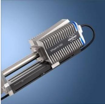
**SEM-EDS:** Analysis based on the sample interaction with an electron beam source from the SEM and the resultant X-rays that are detected using an EDS (simultaneous element detection)
