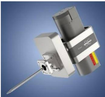
**SEM-XRF-EDS: MicroXRF on SEM (XTrace):** Analysis based on the sample interaction with an X-ray beam source from the Micro XRF attached to the SEM and the resultant X-rays that are detected using an EDS (simultaneous element detection)
