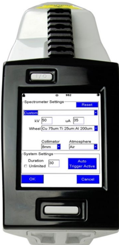
HH Screen for user control of measurement settings
