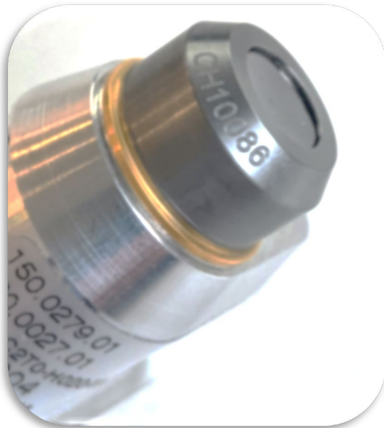
Large area SDD with graphene window
