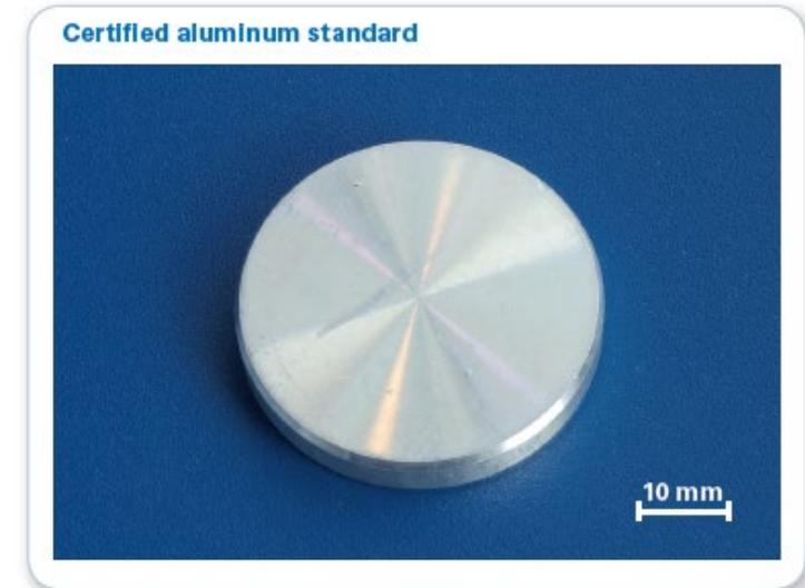
Fig. 1 Photograph of the analyzed specimen Alcoa Deltalloy® 4032
