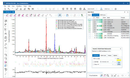
Figure 11 An advanced environmental study demonstrating how automated phase identification with PFRS can be used to fingerprint the mineralogical composition of rooftop dust. The matching mineralogy clearly indicates its origin from Sahara Desert dust events, proving PFRS to be a valuable tool for identifying trace materials in complex environmental samples.
