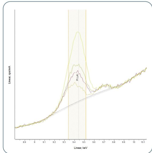
Figure 4: Calibration details. Left: Calibration curve. Right: Overlaid spectra of the standards. The integrated range used for the calibration is indicated in yellow.
