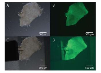
**Fig. 2:** Common brightfield illumination (A) and epi-fluorescence (B) of endothelial aorta tissue. Fluorescent images were collected with a ProgRes CFCool from Jenoptik. In (C) and (D) the cantilever chip can be seen as the AFM head is in place. Sample courtesy of the Institute of Physiology II, University Medical Center Münster, Germany.
