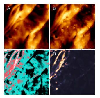
**Fig. 3:** Height image (A), contact point image (B), stiffness (C) and corresponding Young's Modulus image (D) of a mouse skin tissue, using QI<sup>™</sup> Advanced mode. Scan field 6.0 microns. Height z-range 353.3 nm, Contact point z-range 326.5 nm, stiffness z-range 65.6 nN/µm, Young's Modulus z-range 1 GPa. Sample courtesy of Prof. Michael F. Olson, Beatson Institute for Cancer Research, Glasgow University, UK.
