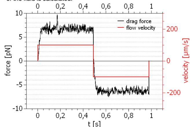
**Figure 2 Viscous drag measurement** in 1:1 glycerol-water mix. The flow of  $100 \mu\text{m/s}$  is generated by moving the sample with a piezo scanner. With a bead of diameter  $d = 2 \mu\text{m}$  the viscosity calculated with equation (1) is  $\eta \approx 3.44 \text{ mPa s}$
