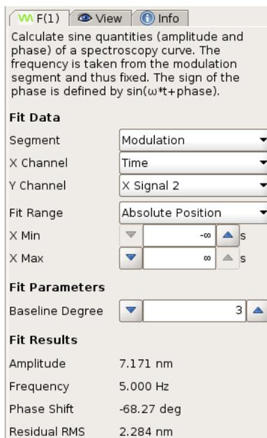
**b) Sine fitting in the NanoTracker™ data processing software.**
