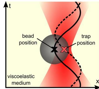
**Figure 7 Trap oscillation method.** The trap position is modulated with a sinusoidal signal which results in a periodic force on the trapped particle. The response (movement) of the particle depends on the frequency of the modulation and the viscoelastic properties of the surrounding material.
