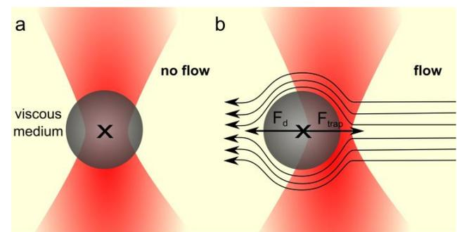
**Figure 1 a)** Principle of a viscosity measurement. **b)** Motion of the fluid surrounding a trapped particle generates viscous drag resulting in the displacement of the particle. The (Stokes') drag force can be measured with high accuracy and with known parameters like bead diameter and relative velocity, the viscosity of the fluid is calculated.
