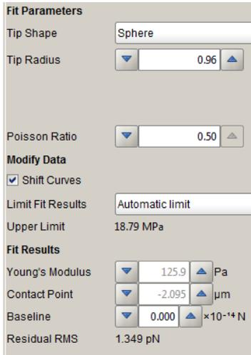
**b) Fit control in the NanoTracker™ data processing software.** With only few intuitive parameters, the force-deformation curve can be approximated with a Hertz fit delivering  $E \approx 125 \text{ Pa}$  for the investigated agarose gel (see equation (2)).
