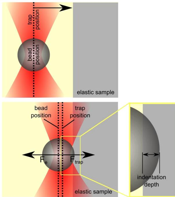
**Figure 3 Indentation Measurement**
