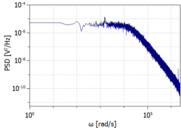
**Figure 6 Power spectral density (PSD)** of a trapped particle's Brownian motion along one direction. The fast electronics in the NanoTracker™ controller allow the detection of particle oscillations up to an angular frequency of  $\omega \approx 2.4 \times 10^6 \text{ rad}$  ( $f \approx 380 \text{ kHz}$ ). For single spectra, frequencies of up to **3.5 MHz** can be achieved.
