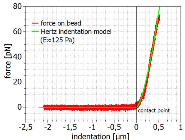
**Figure 4 a) Force-indentation curve of a soft agarose gel.** After the particle has contacted the surface (indentation = 0), the deformation starts. The positive part of the curve was fitted with a Hertz model (green line) to calculate the material's Young's modulus,  $E$ .
