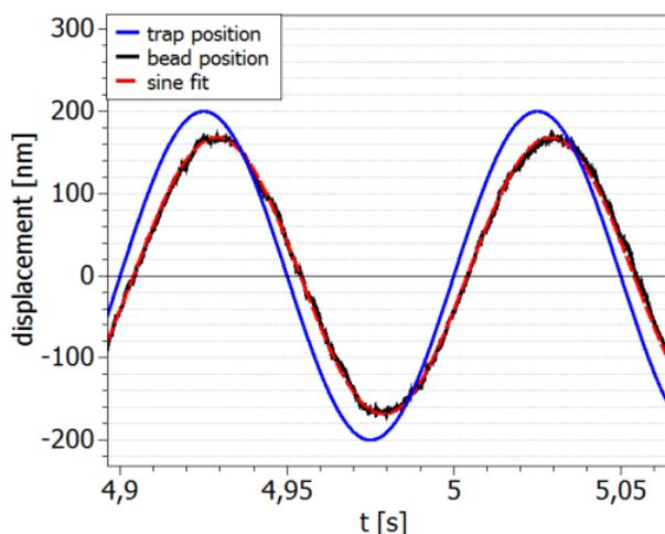
**Figure 8 a) Sinusoidal movement of the trap and the delayed bead response in 1% methylcellulose solution.** In active rheology measurements the trap position (blue curve) is oscillated at different frequencies (here:  $f = 10\text{Hz}$ ). The bead movement is phase delayed due to the mechanical interactions between the particle and the viscoelastic fluid. The red dashed line is a cosine fit to the bead movement that shows a phase delay of approx.  $0.28\text{ rad}$  against the trap position.
