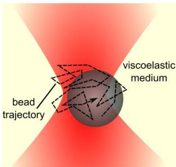
**Figure 5: Passive rheology measurement.** The trajectory of a particle under the influence of collisions with thermally accelerated fluid molecules (Brownian motion) is recorded.
