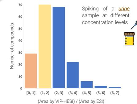
Figure 1: Distribution of 198 detected spiked compounds into groups based on the ratio of the peak area using VIP-HESI source to the peak area using ESI source at  $C_{\text{instrumental}} = 5 \mu\text{g/L}$
