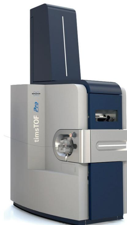
The timsTOF Pro uses trapped ion mobility spectrometry (TIMS), where ions are propelled through the TIMS tunnel by a gas flow. An electrical field controls each ion from moving beyond a position defined by the ion's mobility, where the push it experiences from the gas flow matches the force of the electrical field. Ramping down the electrical field allows selectively releasing ions from the TIMS tunnel according to their mobility.
