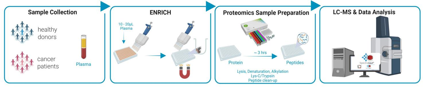
Fig. 1 Complete ENRICH-iST workflow for proteomics preparation of plasma sample in 96-well format
