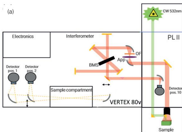
**Fig. 6** Typical configuration for PL measurements including cable connections. (a) Standard NIR PL: measurements with PL II module and purged spectrometer. (b) Vacuum configuration for MIR PL measurement via amplitude modulated step scan.
