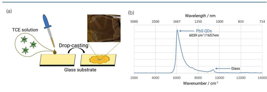
**Fig. 5** Preparation of PbS QDs on the glass substrate (a) PL spectrum in the NIR region of PbS QDs deposited on the glass substrate (b) Spectrum was taken with  $16\text{ cm}^{-1}$  resolution,  $532\text{nm}$  CW,  $80\text{ mW}$  excitation, and InGaAs detector; 16 scans were averaged.
