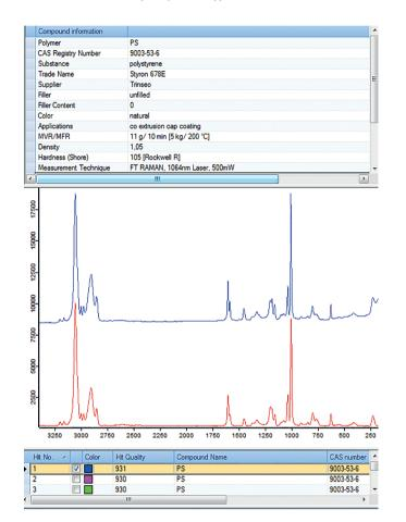
Fig. 1 Result of spectrum identification with the ATR-IR Polymers, Plastics and Additives Library. The upper window shows extensive compound information as well as how the reference spectra were collected.
