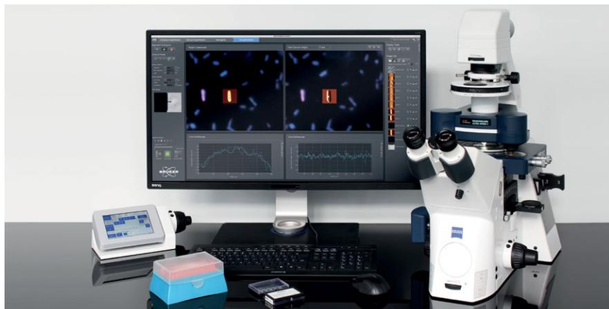
**Morphology:** The new software feature **DynAsyst** and improved **Dynamic PID** enable easy investigation of fragile, unfixed samples at higher speeds and lowest forces.
