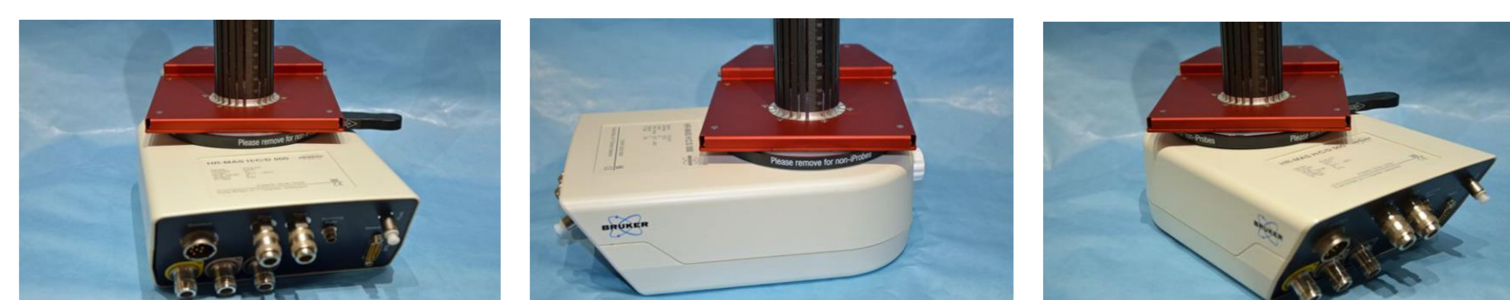
Figure 2: The orientation of the MAS probe to the RT shim system is a parameter of MASshim (left: angle 0, middle: angle 90, right: angle 45).
