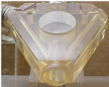
Inertial detection system / gyrolaser
